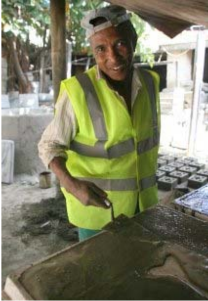
A HIP-trained mason puts the finishing touches on a SanPlat being made in its mold. The finished product (below) is designed to be affordable and easy to clean.
